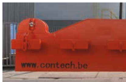
Eye structure for direct crane connection
