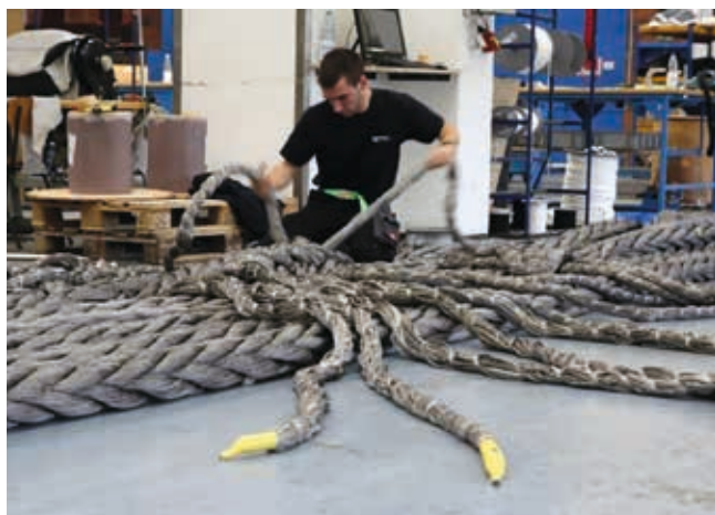
Beyond the limits: a megasling with 900t WLL being custom made
