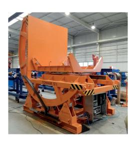
Tilt tables can be used to rotate loads other than sheet coils, such as forms, welded parts, fitting... Work surfaces can be plastic coated to prevent damage to the load. The cradle can be equipped with holding arms for gripping pallets, narrow coils. The load area can be sliding, rotating or equipped with a roller conveyor according to the customer's requirements. The table can be supplemented with a service platform or embedded in the floor. Rotation can be realized by up to 180°.
