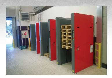
1-5 pallets can be taken to the machine at the same time for automatic stacking or, conversely, 1–5 pallets can be taken off the machine at the same time at floor level.
