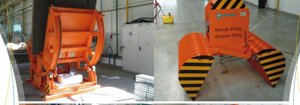
They serve for handling of materials like coal, sand, wood chips etc. Volume and load-bearing capacity of the dipper depend on the volume of transport (m3/hour), crane capacity and other factors.
