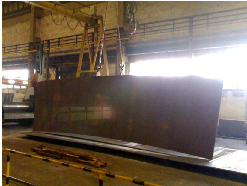
Vertical transport of various plates
