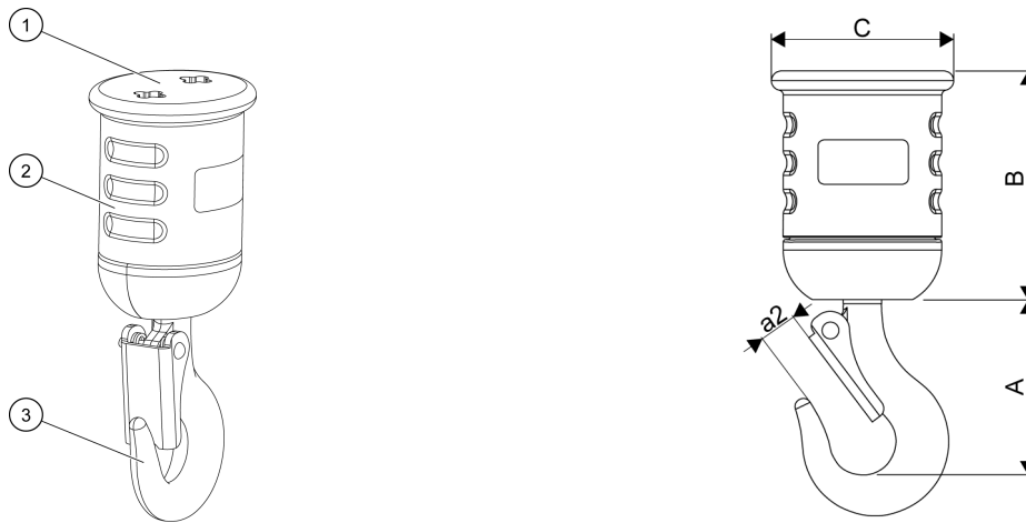
Figure 28. Two-fall (2/1) hook block for frame sizes 02–05
